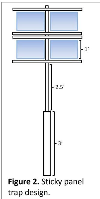
**Figure 2.** Sticky panel trap design.
