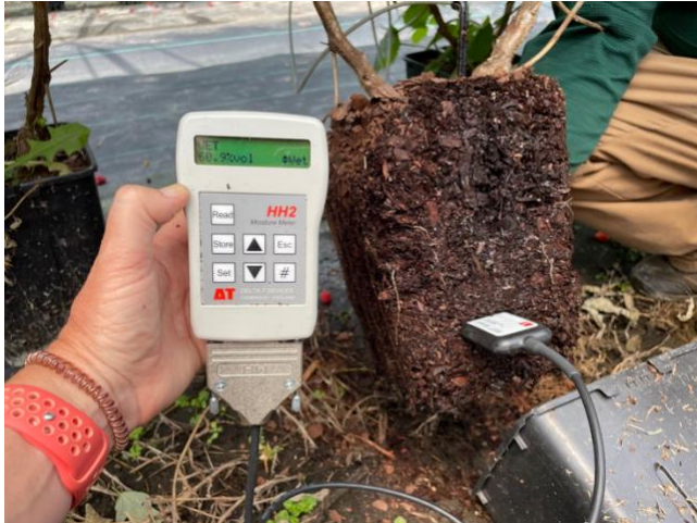
Monitoring substrate moisture and EC using the WET-2 sensor.
