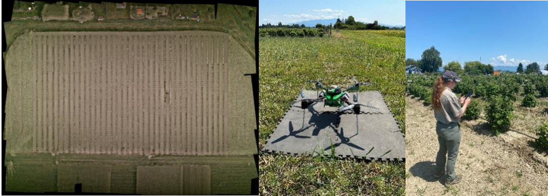
Figure 3: Left: Constructed orthomosaic of aerial images taken May 5 th , 2023. Constructed by Alexander Gregory. Middle: The AgBOT mk 1 quadcopter equipped with a MicaSense RedEdge-MX multispectral sensor and the FLIR Vue R thermal sensor. Photo by Savannah Phipps. Right: Savannah Phipps recording images of select genotypes using the AgerPoint Capture app on the iPhone 14 Pro Max. Photo by Hannah Baker.
