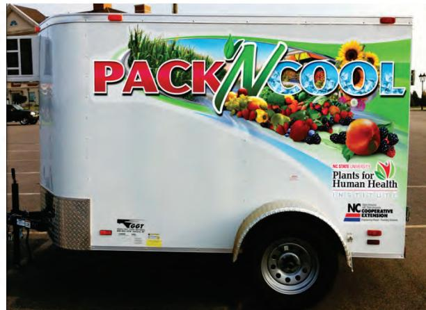
Conversion of a 5 x 8 cargo trailer, barn door style, 3800 lb load capacity, to the Pack N Cool refrigerated trailer by adding an AC unit, a cool bot to make it run cold ([storeitcold.com](http://storeitcold.com)), insulation, and a 110 volt receptacle with a 14 gauge 50 foot extension cord.
