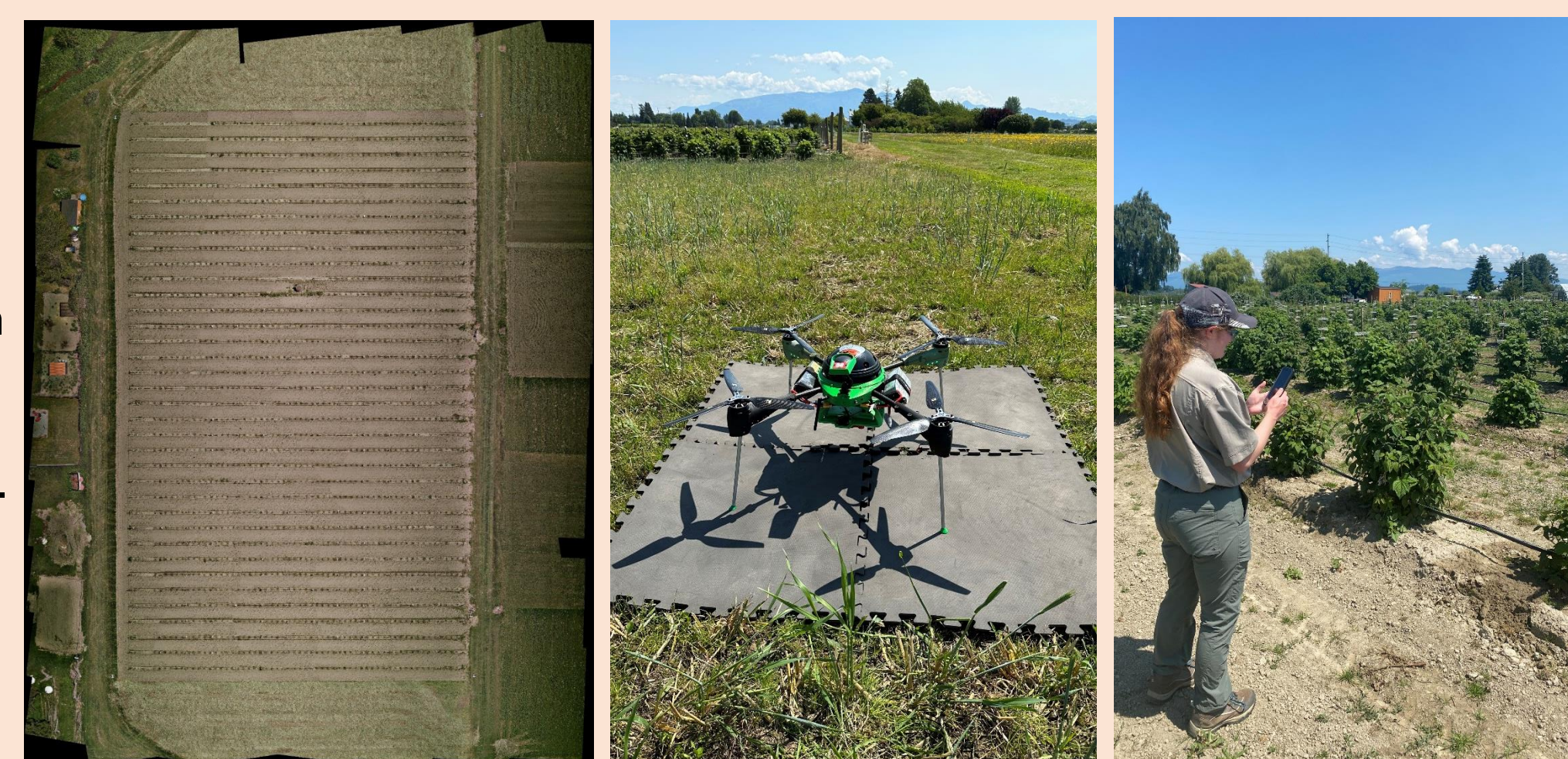
Figure 7 (right): Examples of ground-based and aerial imaging in action. A) Stitched red-green-blue aerial orthomosaic of field trial from May 5, 2023. Photo by Alexander Gregory. B) AgBOT mk 1 Quadcopter equipped with MicaSense RedEdge-MX multispectral sensor. Photo by Savannah Phipps. C) Savannah Phipps imaging in the AgerPoint Capture app with iPhone 14 Pro Max. Photo by Hannah Baker.
