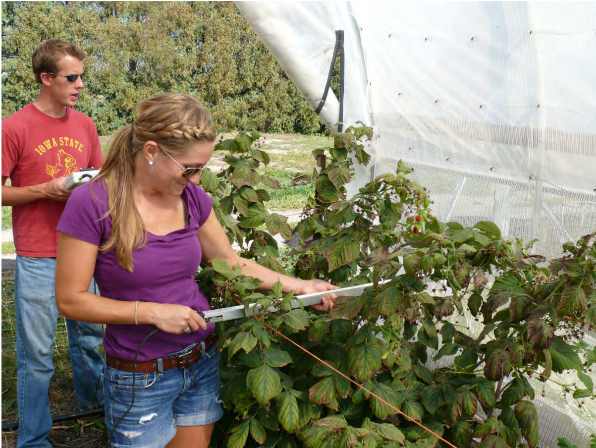
Photo 2: Leah Riesselman (graduate student) and Austin Schott (student intern) recording light transmission through canopy irradiance.
